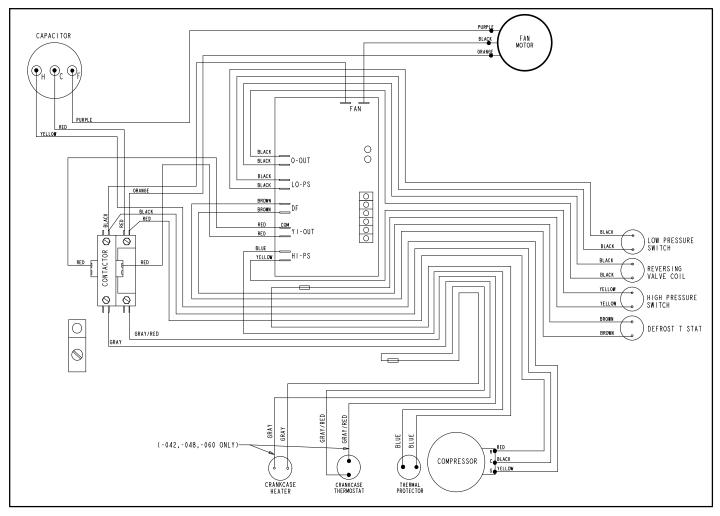
Figure 15. Typical Factory Wiring
